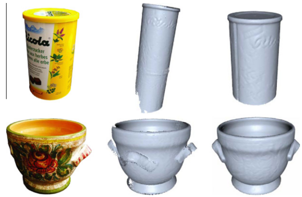
Fig. 11. Modeling results for textured objects. The middle column shows the artifacts that arise due to symmetries when only geometry is used for registration. The right column shows the correctly reconstructed objects when texture features are used for registration.
