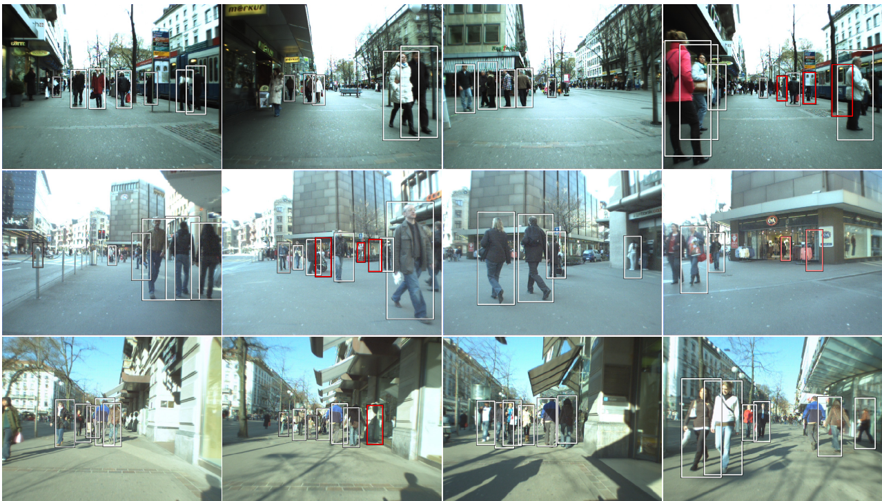
Figure 11. Experimental results obtained on 3 test sequences. Note the level of interaction between pedestrians (frequently overlapping bounding boxes). The images also show some typical false positives in red (trees, children's stroller, signs, mannequin).
