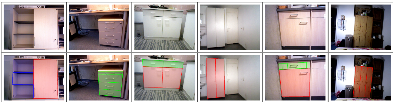
Figure 5: Qualitative results: The input real Kinect images and corresponding segmentation are displayed respectively on row 1 and row 2. Columns 1-5 shows the success cases while columns 6 displays the failed cases. The two main reasons for failure are missed edges and high amount of texture. (door, drawer and shelf).
