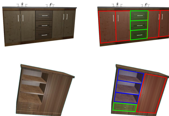
Figure 1: Semantic segmentation of modular furniture in RGBD images: Left column is the input front face of the furniture and right column is the segmentation output (door, drawer and shelf).
