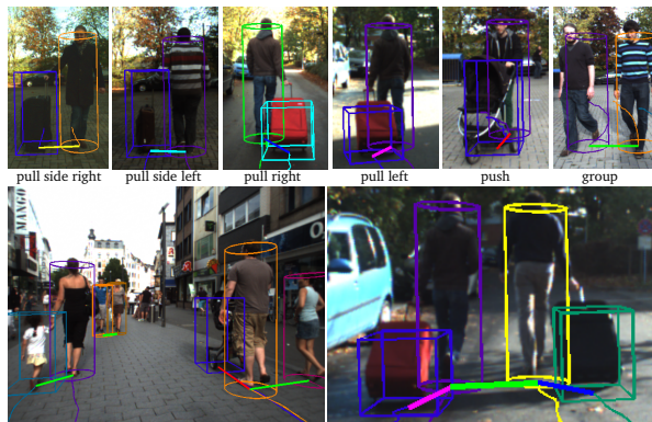
Figure 1: Our proposed approach models pairwise interactions between persons and objects in a probabilistic graphical model, taking into account object shape, relative arrangement, and temporal consistency. Thus, it can infer which objects belong to which persons and predict how the interactions will continue. Recognized interactions are visualized by colored lines linking the foot points of interacting objects (Legend: pull side right , pull side left , pull right , pull left , push , group ).
