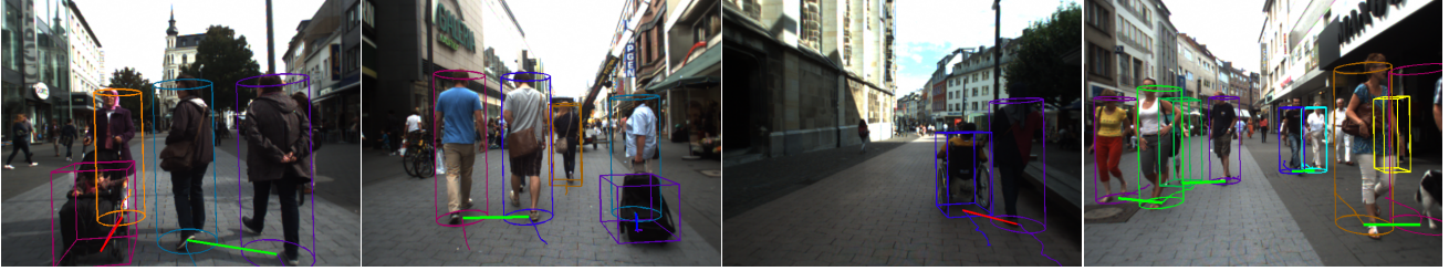
Figure 9: Result images showing tracked persons and their associated objects with correct action inference. Interactions are visualized by linking the footpoints of the interacting objects by a colored line. Green -group, red -push, blue -pull right, magenta -pull left.
