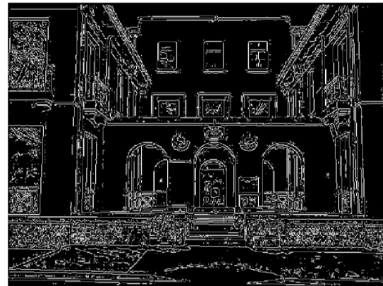
Low threshold (weak edges)
