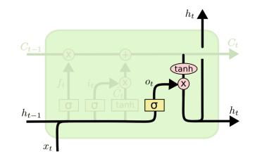
$$o_{t} = \sigma \left( W_{o} \left[ h_{t-1}, x_{t} \right] + b_{o} \right)$$
