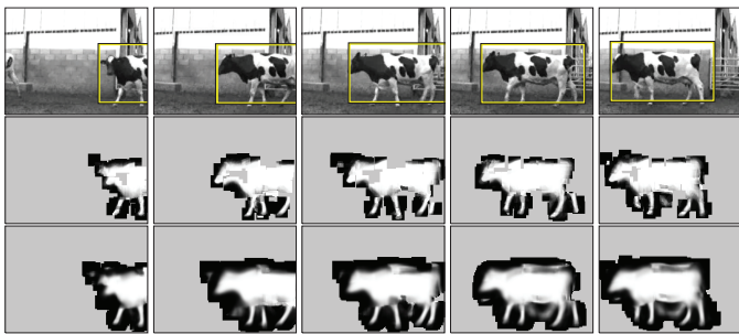
Fig. 21. Example detections and automatically generated segmentations from one cow sequence. (middle row) segmentations obtained from the initial hypotheses; (bottom row) segmentations from refined hypotheses (with additional features sampled in a uniform grid).
