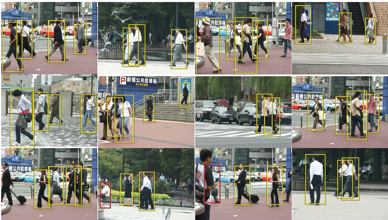
Fig. 23. Example detections of our approach on difficult crowded scenes from the TUD Pedestrian test set (at the EER). Correct detections are shown in yellow, false positives in red.
