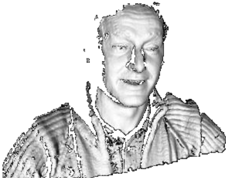
Dense 3D reconstructions at 30 fps (on the GPU )
