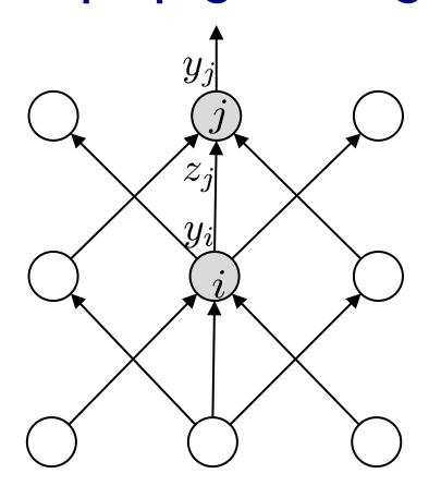
$$\frac{\partial E}{\partial z_j} = \frac{\partial y_j}{\partial z_j} \frac{\partial E}{\partial y_j} = y_j (1 - y_j) \frac{\partial E}{\partial y_j}$$
