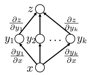
$$\frac{\partial z}{\partial x} = \frac{\partial z}{\partial y_1} \frac{\partial y_1}{\partial x} + \frac{\partial z}{\partial y_2} \frac{\partial y_2}{\partial x} + \dots$$
